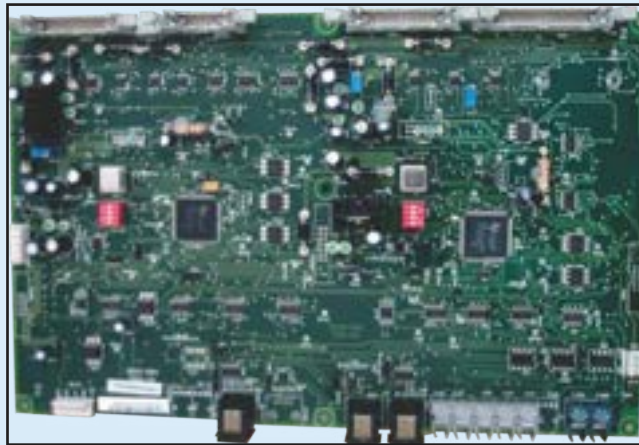
Digital Signal Processing (DSP) based control board
