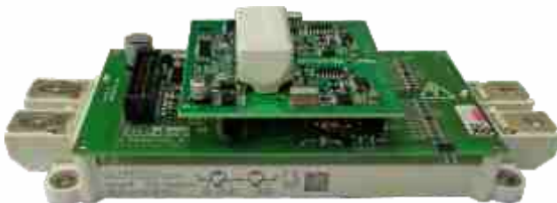
IGBT modules in inverter
